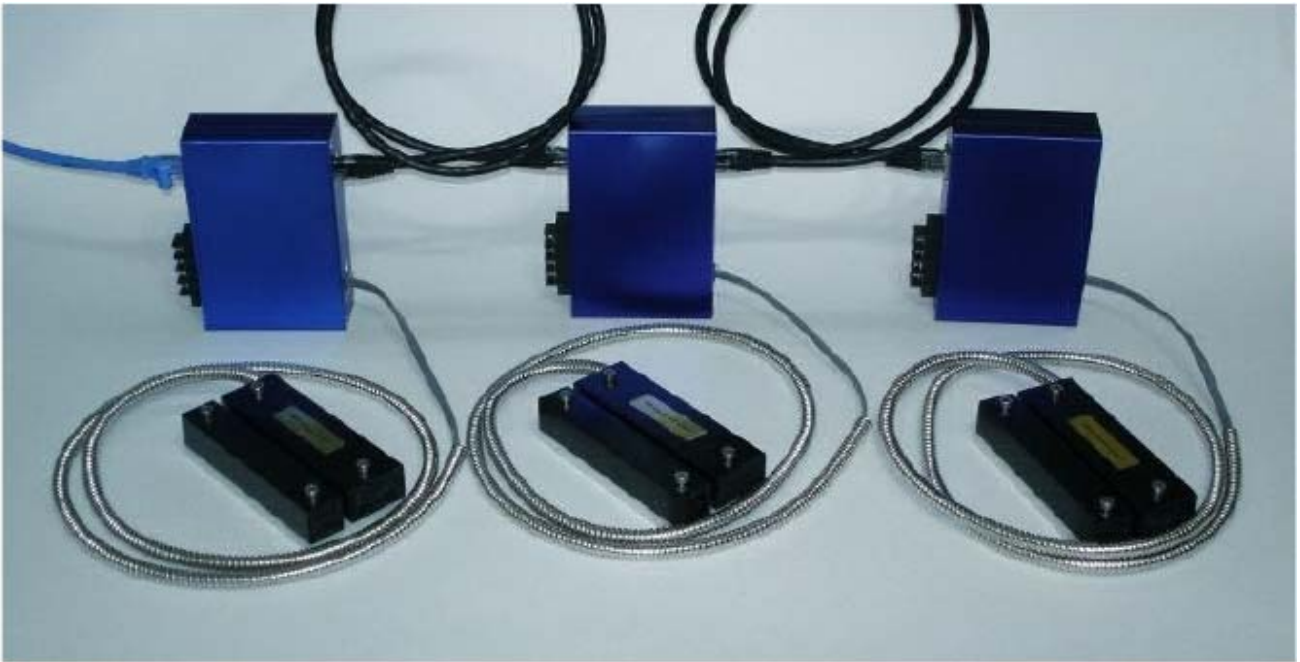
Three switches of the 3D Magnetometer network type connected as nodes on an RS485 network.
