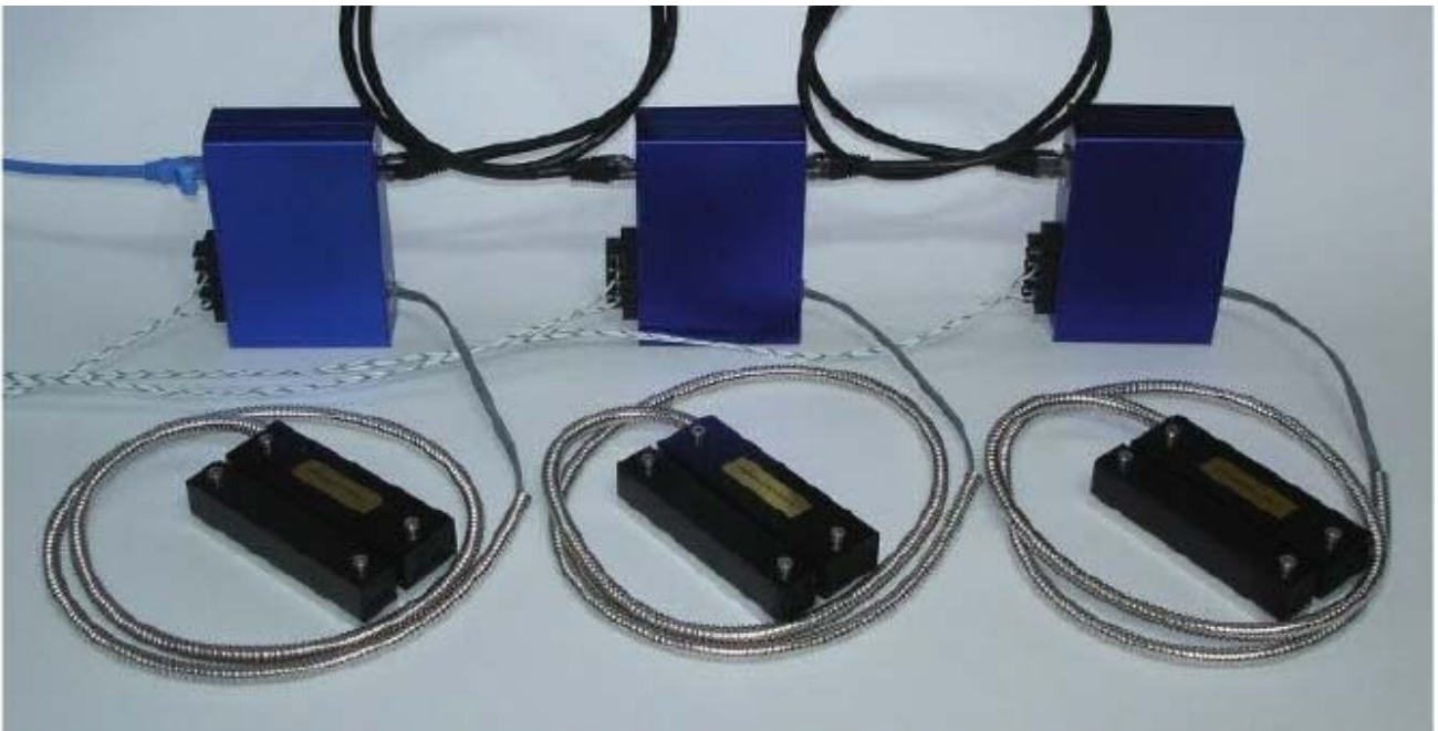
Three switches of the 3D Magnetometer network type connected as nodes on an RS485 network and to a conventionally wired system in parallel. This configuration uses an existing installation without modification and allows a network to be built up on top of it with a string of Ethernet cables. Remote test can be initiated from either system without collisions and register correctly on both systems simultaneously. Any existing system can be upgraded one node at a time.
